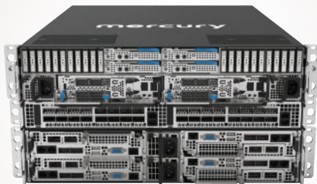
The Rugged Data Storage (RDS) system from Mercury Systems helps give fast and secure access to big data, AI, and machine learning at the edge aboard naval vessels.
